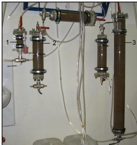
Figure 1: Filtration columns: 1 – length 10 cm and diameter 40 mm, 2 – length 30 cm and diameter 70 mm, 3 – length 110 cm and diameter 80 mm.
